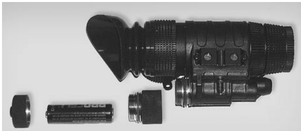
Figure 4-2 DNAAS Battery Installation.
